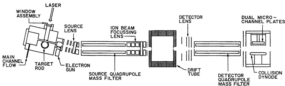
Fig. 1 Schematic diagram of the injected-ion drift-tube apparatus
